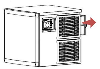
⚠ Note: Be careful when doing the condenser cleaning as the edges of the fins are sharp.
